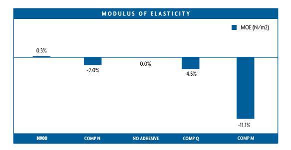
In terms of Elasticity, N900 improved the Modulus of Elasticity as compared to all competitive adhesives. Indeed N900 was the ONLY adhesive that improved the elasticity of the samples. All other adhesives reduced the elasticity compared to the control samples made without adhesive.
