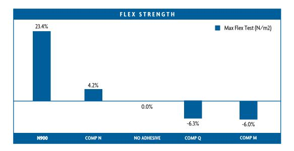
In tests per ASTM D790, independent laboratories\* found N900 improved the strength of samples almost 20% and 30% compared to competitive adhesives. In fact, N900 samples were found to be even stronger than samples made without adhesive.
